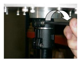
Figure 7. Securing the platform to the support.
