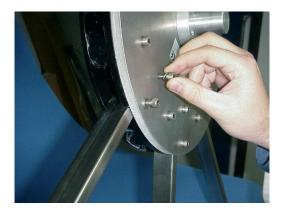
Figure 4. Screwing the Allen screws
