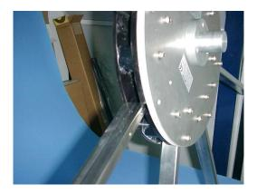
Figure 3. Inserting the arm in the circular base
